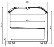
For version AD/U the inner dimensions are reduced due to the necessary use of wire grids along the inside walls.
